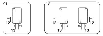
If there is more than one opening contact, they must be connected in parallel (see picture 2).
