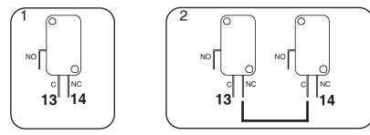
① If there is more than one stop contact, they must be connected in series (see picture 2).
